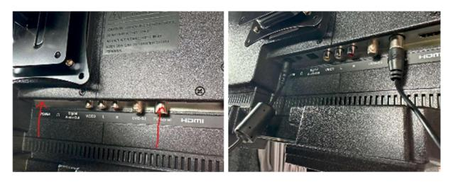
Plug the power lead in to the 12v socket and then into the underside of the TV as shown below. Plug the aerial in to the "TV aerial".
