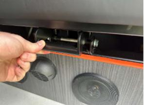
Next pull the seat belts out as shown and start to slide the seat base forward. The whole seat will now start to slide and move towards the flat position.
