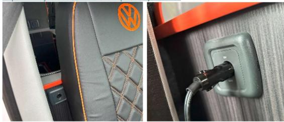
The TV requires the power lead to be fitted. The 12v power socket for the TV is located in the end panel of the sink unit on the end behind the driver's seat.
