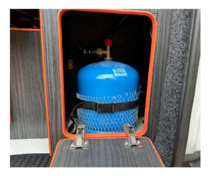
Pull down the hatch to reveal the gas cannister. The hinges are spring loaded so please lower the door carefully.
