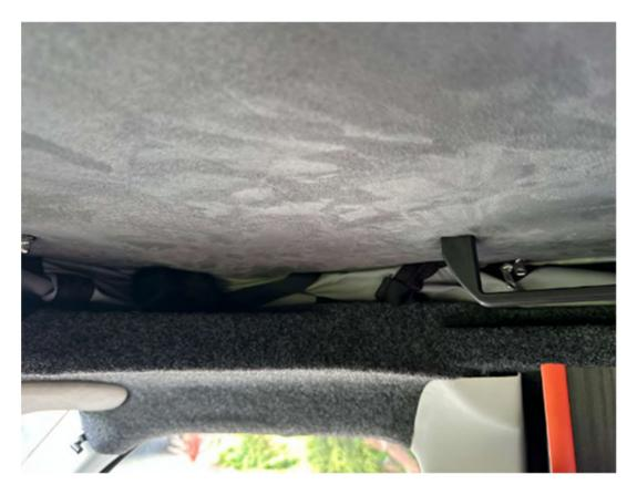
Carefully tuck the excess roof material in around the roof internally.
