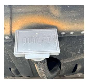
Locate the grey wastewater outlet on the underside of the driver's side of the vehicle in front of the rear wheel.
