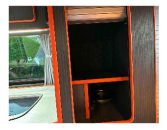
There is a large storage compartment next to the sink area – this is opened by lifting up the tambour door to full height – the door will not stay open part way, it must be fully opened. This compartment generally houses the cooking and dining equipment. Please be careful when closing the door not to drop down the sliding door – please lower carefully.
