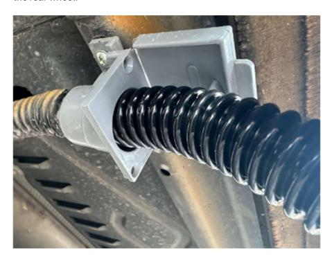
Carefully lift the grey flap and connect the short black ribbed waste pipe. The pipe is stored in the rear storage compartment of the vehicle under the rear seats.
