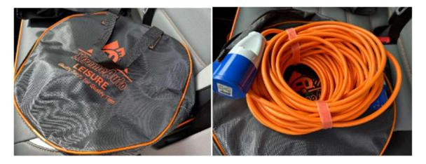
Connect the lead to the vehicle first using the female adaptor end. This is so you are not carrying a live unconnected cable. Unroll the cable completely and connect to the electric hookup point. Important – do not leave the cable tightly coiled up when connected as it can potentially overheat.
