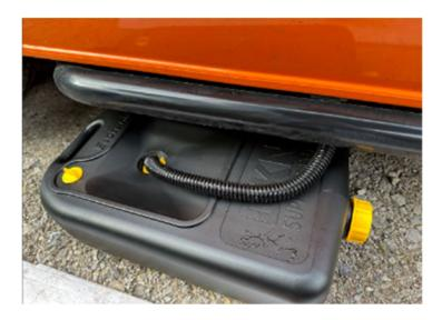
Unscrew the large yellow cap from the dished section of the tank. Please keep this cap safe in the vehicle, if left outside it may be blown away. Place the black wastewater container under the vehicle and lay the ribbed pipe into the receptacle. The tank is stored in the rear storage compartment under the rear seats accessed from the rear barn doors.
