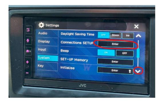
Press the down button on the touch screen once until the **"connections setup"** item appears. Press enter.
