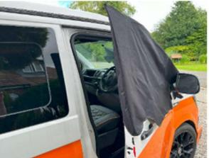
Then spread the cover over the front windscreen around to the other door and hook over the second door – due to the snug fitting of the cover ensure the first door is shut and the second door is only slightly open just enough to hook over the cover.
