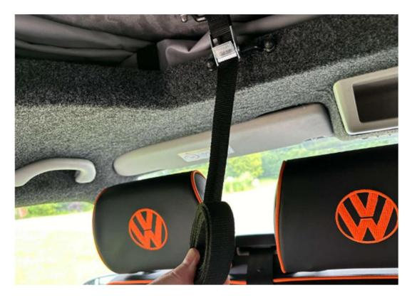
These two straps and clips are the only thing holding the roof closed so please make sure they are secured and under tension.
