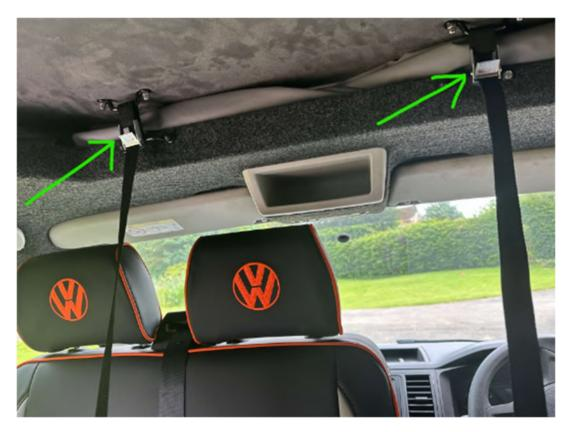
The two black strap and clips above the cab secure the roof down. Release the two crocodile clips and pull out the strap. Do not fully remove the strap but allow enough slack for the roof to rise.
