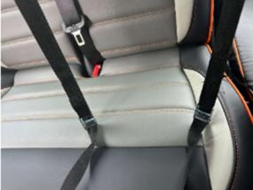
If you pull the crocodile clips down on the strap until they are sat on the passenger seat this will give you sufficient slack to raise the roof.
