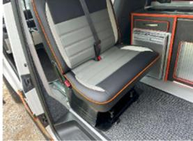
Keep turning the seat anti-clockwise until facing the rear of the vehicle. Now the seat can be pushed backwards and forwards as required for seating or dining. It can help to slide the seat slightly towards the passenger side of the vehicle to avoid hitting the handbrake.
