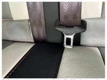
Quite often the seat belt clips will slide down and remain under the seat base – to retrieve these just push your hand in to the gap and slide the clips back up ready for use.
