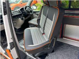
The easiest way is to push the seat straight back towards the rear of the vehicle and then rotate anti-clockwise – at this point be careful to avoid the TV (if fitted) and the handbrake.
