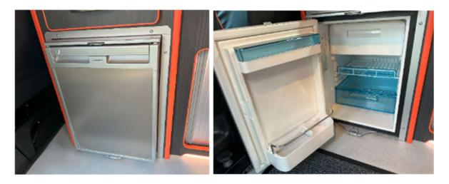
To open the fridge door, lift up the handle located at the top – grip the handle to the right hand side of the fridge.
