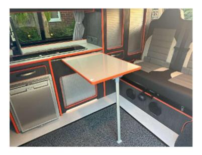
Locate the table on to the rail on the face of the unit just below the sink with the two clips and lower the support leg. This will require the table to be angled down slightly to engage the hooks, lift the support leg slightly to help with this manoeuvre.
