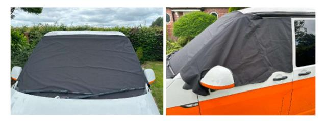
Once in position on the second door ensure the cover is fitted neatly over the windscreen and close the second door. Now tuck the cover under the windscreen wipers and secure around the two wing mirrors with the Velcro straps.
