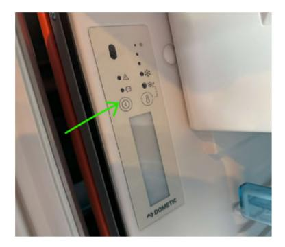
To turn the fridge on, press and hold the power button shown above. To turn the fridge off, press and hold the same button until all the lights go off. The fridge can be operated without the leisure battery switched on so you can cool food and drinks while driving to your destination.
