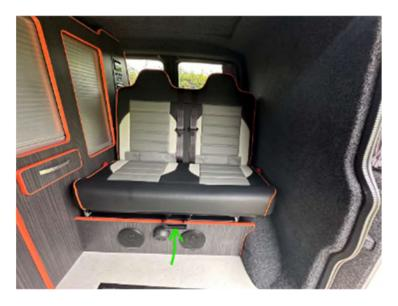
To convert the seats to a bed, lift the release handle located under the base of the seat as shown.
