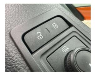
When locking the vehicle on a night do not use the key remote fob – this will activate the alarm and movement sensors. Lock the doors using the central locking button in the front cab located on the driver's door.
