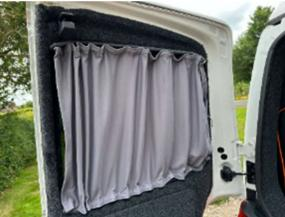
The curtains have small runners top and bottom that slide across within a metal track to open or close the curtains. These can be fiddly sometimes so please be careful – try to slide the top and bottom together to make opening and closing easier. If the runners catch in the track they can be wiggled back and forth gently to help them move.
