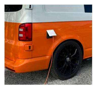
Where electric hookup is available connect to the vehicle. The connection point is on the driver side of the vehicle located towards the rear under a plastic flap.
