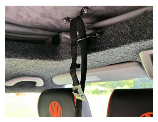
The roof is now secured down using the two straps and crocodile clips. Make sure theses straps are pulled down to create tension and the roof sits snug down to the van.
