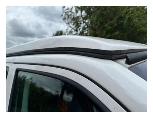
The final check is to ensure the pop top roof is set down flush on the vehicle roof. This is very important – if the roof is not sat flush and tight to the roof and fully secured there is a danger that when driving at speed the wind could force the roof up and cause a major incident.
