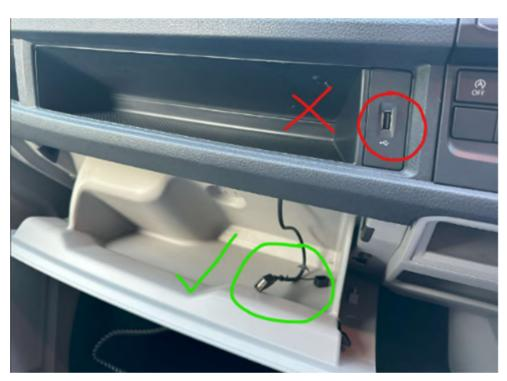
Please use the USB charger located within the glove box compartment. The USB port mounted on the dashboard is not connected and will not work.
