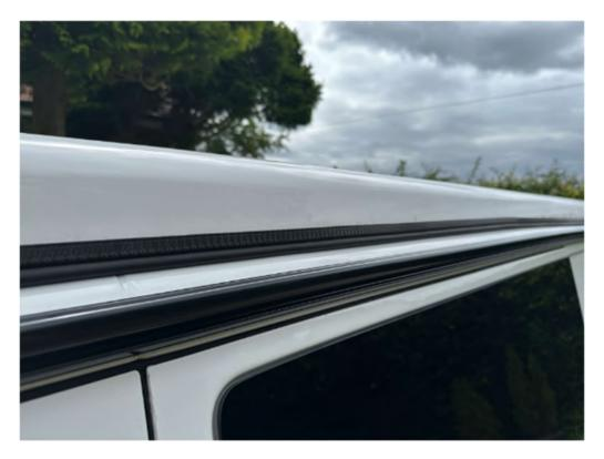
Check externally that there is no roof material trapped between the pop top roof and the van roof. If there is, lift the roof up again and repeat the previous steps ensuring the material is not trapped.
