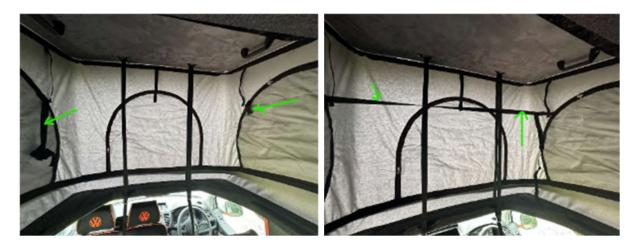
The lateral restraint straps help pull the pop top roof fabric inwards when closing the roof. Once the roof is closed the front lateral restraint strap can be disconnected and the straps tucked in.
