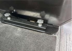
The seat is secured by five sprung screws, three to the rear and two to the front, which screw into the chassis.
