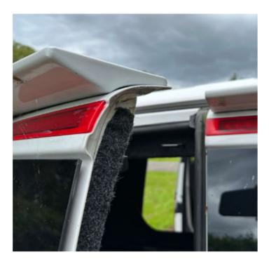
When closing the two rear barn doors always ensure the right hand door (Viewed from the outside) is fully closed before the left hand door. If the doors are not shut in this manner the roof spoiler and paintwork will be damaged.
