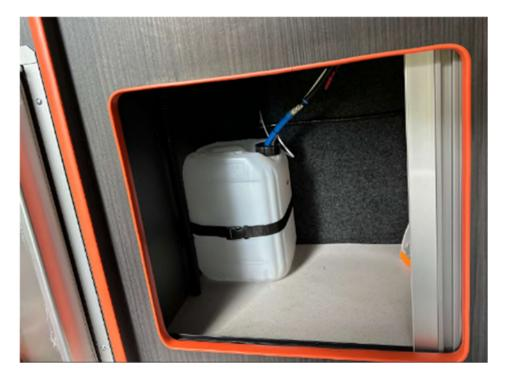
The freshwater tank to supply the sink is located in the cupboard underneath the sink.
