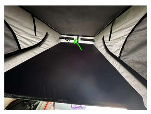
Stand in the van facing the rear and pull down the bed platform first. This is on gas struts so will be easy to pull down. The rear lateral restraint strap is shown by the arrow above. The lateral restraint straps help pull the pop top material inwards when closing to help prevent it becoming trapped between the roof and the vehicle once closed.
